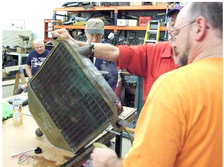
The bad news was that the bottom had been replaced with a steel pan in the past and had rusted to the point that the radiator could not be repaired.
