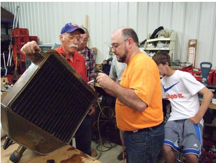
The bad news was that the bottom had been replaced with a steel pan in the past and had rusted to the point that the radiator could not be repaired.
