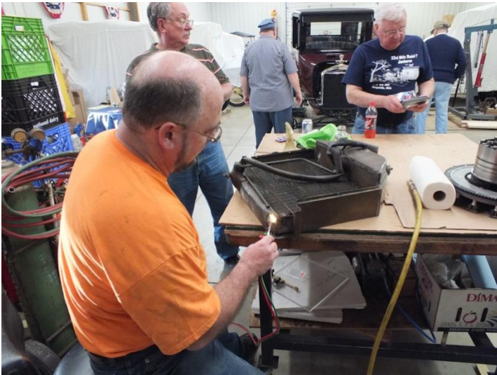
The second demonstration was Jim Cook showing how to patch a brass radiator.
