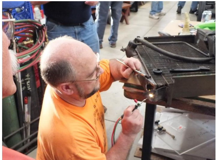
The second demonstration was Jim Cook showing how to patch a brass radiator.
