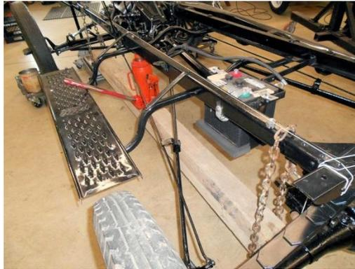
*I elevated the string, at both ends, above the chains. Then the height of the string was measured at the elevated point. The amount of sag was determined by checking the increase of the distance from string to frame along the length of the frame side.*
