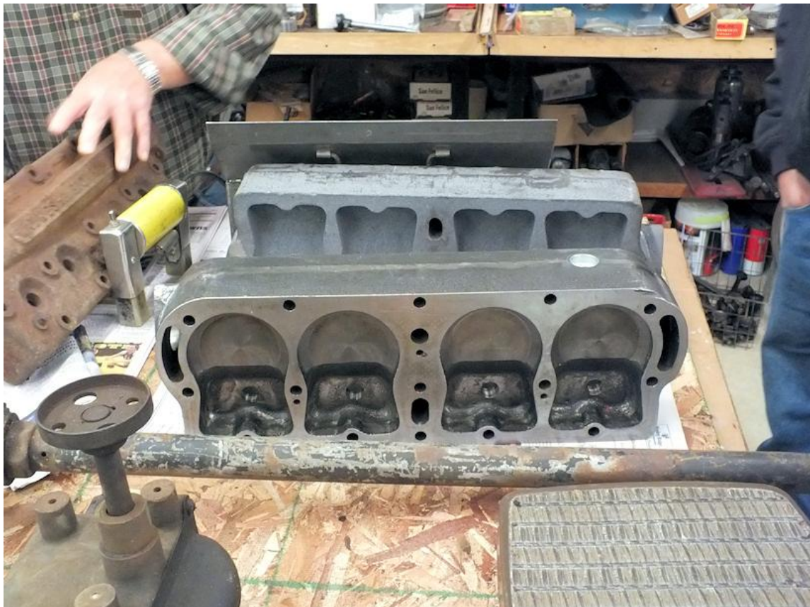
Head in the foreground is machined. One in the back ground is un-machined.
